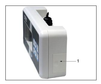
Open the battery compartment cover (1) at the base of the display unit and insert the rechargeable battery. Charge the rechargeable battery for at least 12 hours before initial use.
