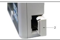
Insert the batteries into the battery holder
